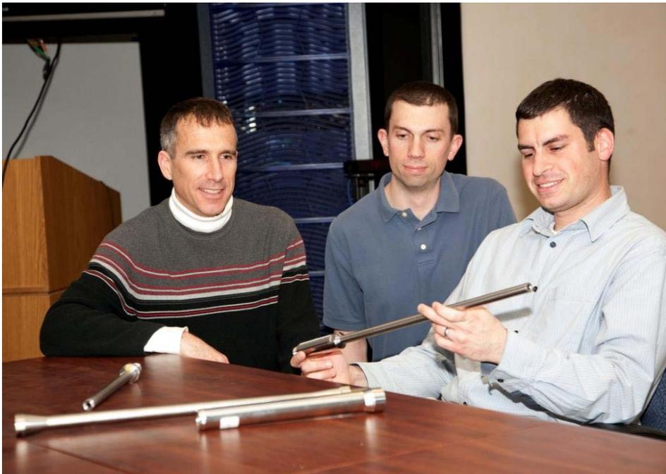
*Far right, engineer Vinny Leto holds one of the various cobalt alloy barrels produced using the flow forming technique. The shortest barrel was the first produced, followed by full length barrels without rifling and later a prototype with rifling like the one that was tested. Other team members, from left, Michael Hespos and Keith Koehler.*
