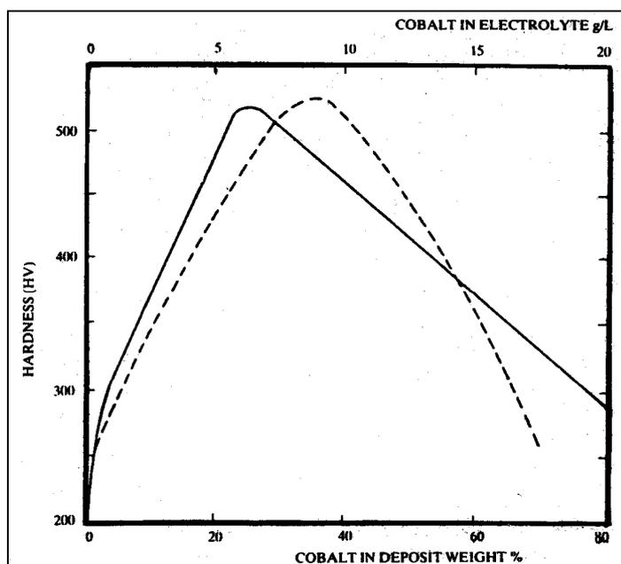
Figure 1 – Hardness of an Inco Co-Ni deposit in relation to the cobalt content of the deposit (---) and the cobalt concentrations in the electrolyte (-)
