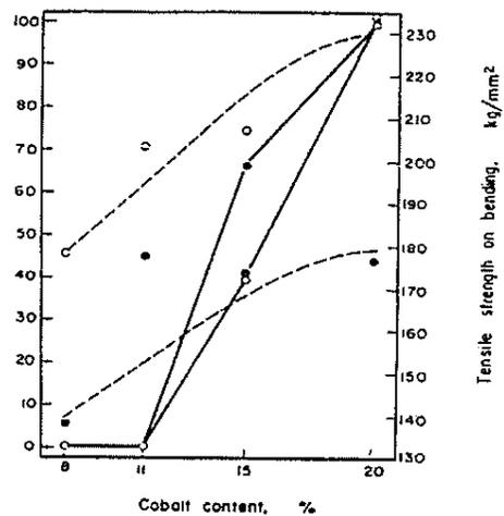
Fig. 3 – Relationship between strength & cobalt content for VK hardmetals produced from tungsten reduced by hydrogen at 650-820°C, with ordinary and intensive grinding of the mixtures
