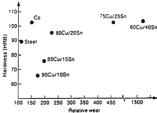
Fig. 1 – The relationship between wear resistance and hardness of bronzes and some metals. Results are relative to a wrought mild steel specimen (= 100)
