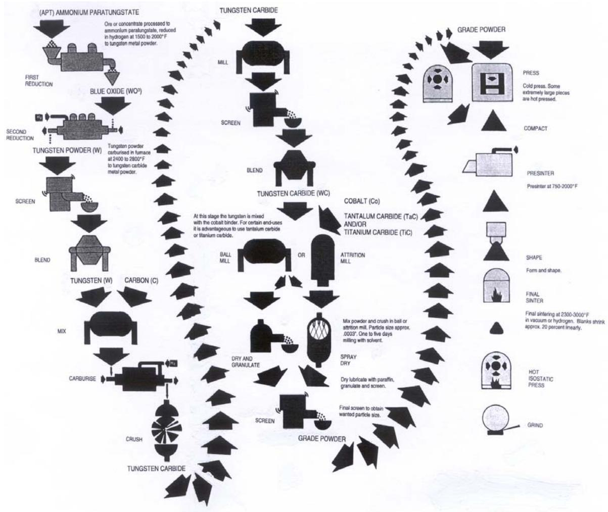
From the original binary carbides, many other mixed carbides have developed – NbC, TaC, TiC, Cr<sub>3</sub>C<sub>2</sub> – all aimed at giving certain properties allied to specific applications. More recently cutting tools have been coated with TiC to further improve cutting speeds (other coatings used are TaC, TiN, TiCN).
