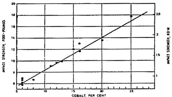
Fig. 2 – Effect of composition on impact strength of WC-Co alloys having a WC grain size from 1.4 to 3.1 microns
