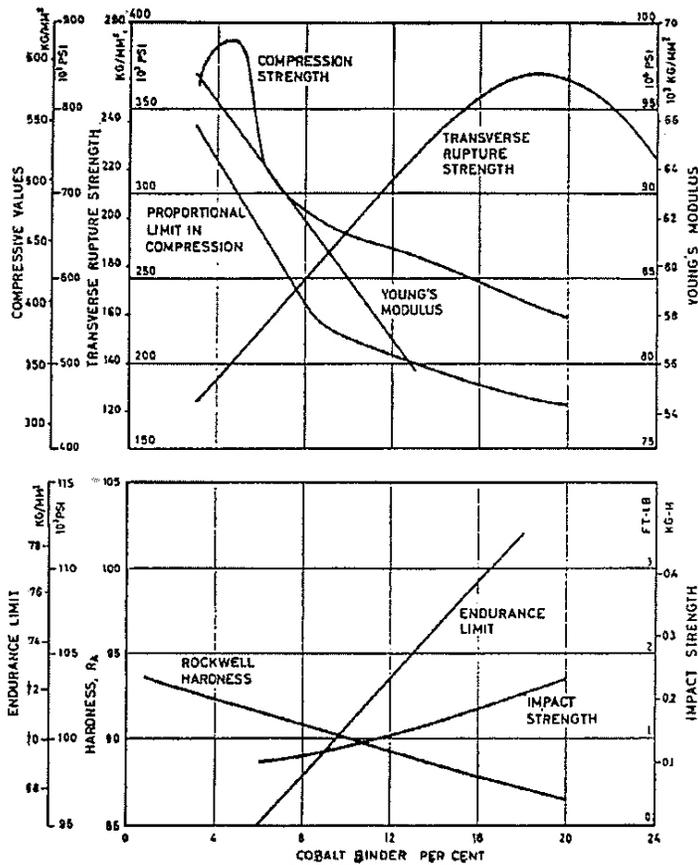
Fig. 1 – Variation in mechanical properties of straight tungsten carbide of normal particle size as the relative amount of cobalt increases
